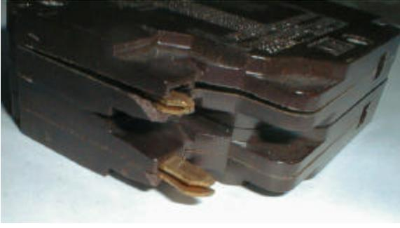
*Figure 8 – Damaged “E” type breaker*
